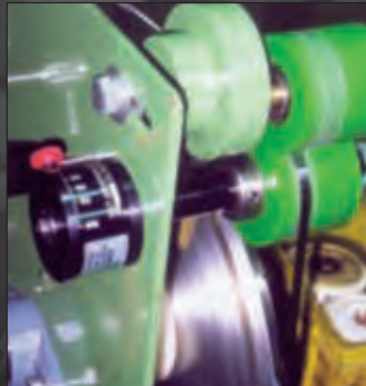
Tensioning films & foils. Model 527 with urethane "nib" roller.
