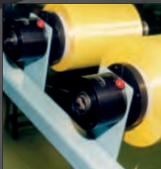
Tensioning Aramid Yarn using Model 523 with Spiked Drive Plate Assembly #750-034.
