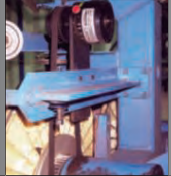
Retrofit application using Model 523 and 700-002M Mounting Bracket on Twister.
